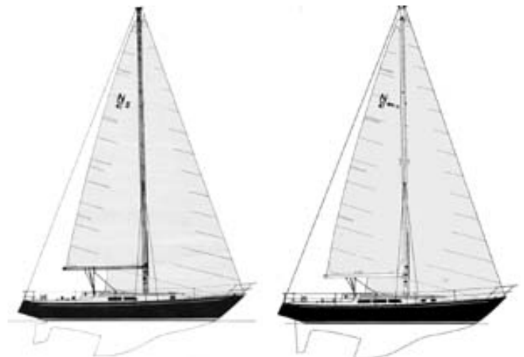
These profiles of the Mark I and Mark II versions of the Newport 41 show slightly different underbodies and portlight design. The rudder change on the Mark II added two feet of waterline length.
